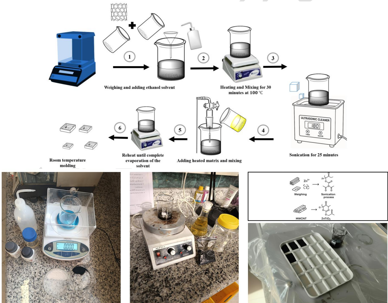
Fig. 4. Experimental procedure for laboratory-scale nanocomposite fabrication
